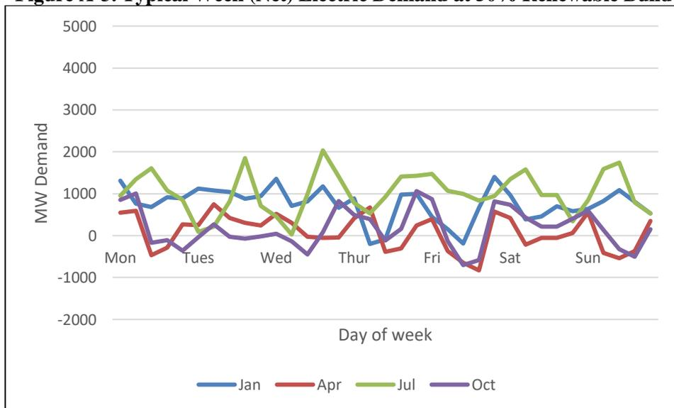
Figure A-3 indicates average demand for all seasons has decreased greatly and the recurring feature of daily demand profiles shown in Figure A-1 has been replaced by non-recurring variability to different degrees; this effect can be
